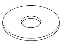
$\varnothing 6/\varnothing 18$  mm
